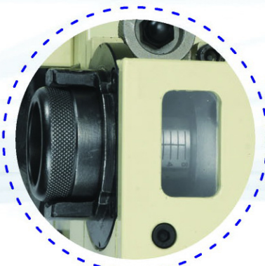
調整切削力裝置 The device with drilling force adjustment
